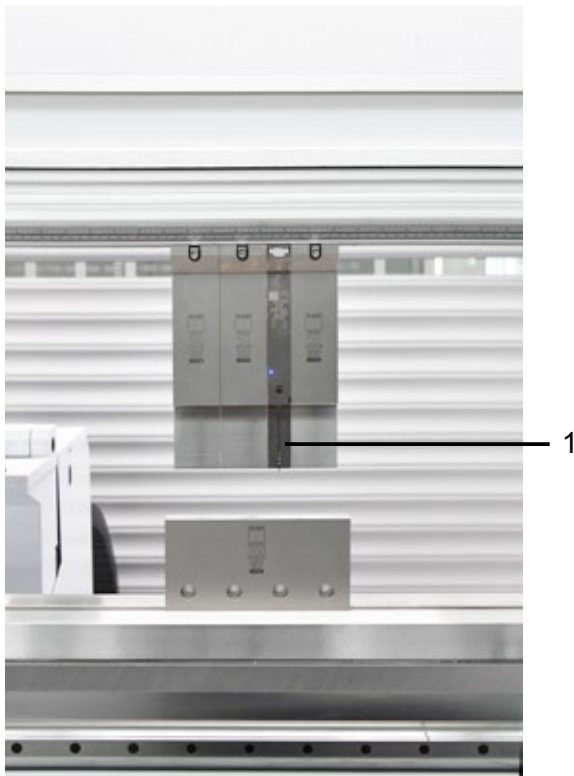
ACB Wireless angle measuring system TruBend Series 5000 (B23), 3 rd generation, TruBend Series 7000 (B28)
